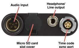
The audio input circuitry is the essentially the same as on Lectrosonics SM and L Series transmitters. Any microphone wired as Lectrosonics "compatible" or "servo bias" will work with the PDR. See page 10 for details.
