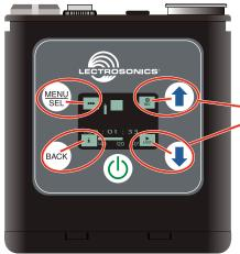
Functions indicated by the icons on the LCD are activated by pressing the adjacent buttons on the keypad
