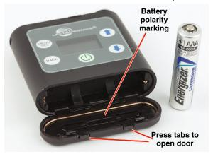
Insert the battery according to the markings inside the battery compartment door. The (+) pos. end of the battery is oriented as shown here.
